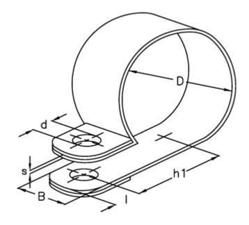
$\begin{array}{ll} d & = 5.3 \\ \text{Diameter D} = 69 \\ \text{h1} & = 41.3 \\ \text{I} & = 5.0 \\ \text{s} & = 0.5 \\ \text{Width B} & = 12 \\ \end{array}$
